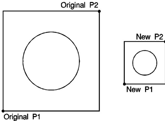
**Figure 19-4 Changing the size of a drawing**
