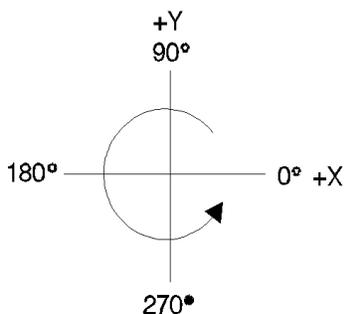
**Figure 22-6 Positive Angle of Rotation**
