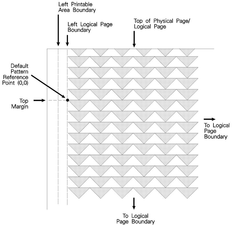
**Figure 13-7 Pattern Layout Across the Printable Area**
