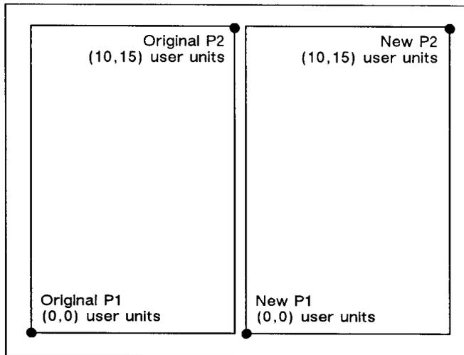
**Figure 19-5 Drawing equal-size pictures on a page**
