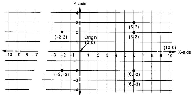
**Figure 17-4 The HP-GL/2 Coordinate System**
