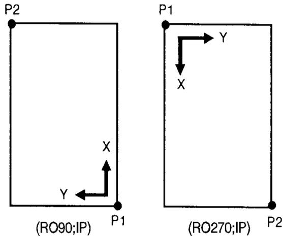
**Figure 19-16 Using IP after the RO Command**
