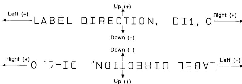
**Figure 23-12 Interaction of Label Direction and Parameter Sign**
