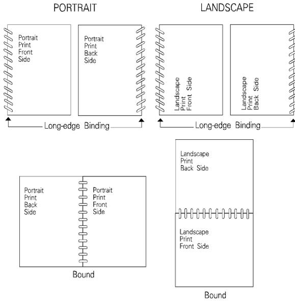
Figure 4-2 Long-Edge Binding Mode
