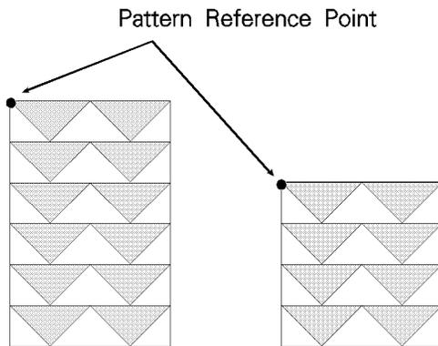
**Figure 13-8 Moving Pattern Reference Point for Pattern Filling**
