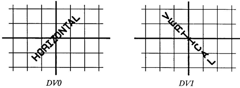
**Figure 23-16** Effect of Horizontal and Vertical Text Paths
