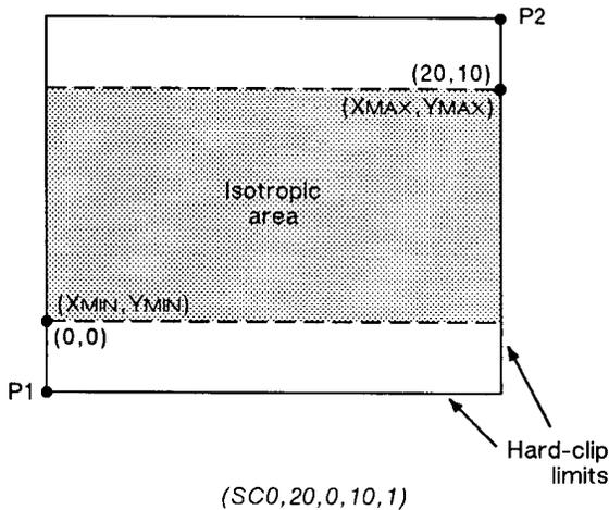
**Figure 19-18 Isotropic Scaling**
