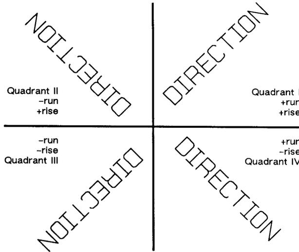
**Figure 23-24 Varying Print Direction with DR Command Parameter Sign**
