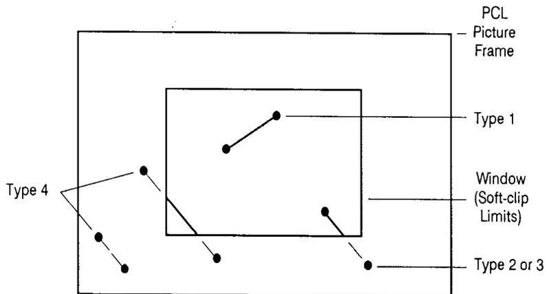
**Figure 19-8 The four types of line segments**
