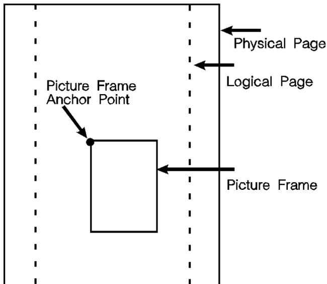
Figure 2-3 PCL Logical Page with HP-GL/2 Picture Frame
