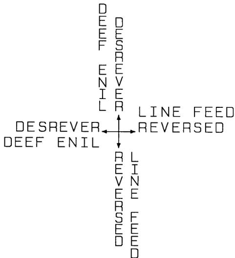
Figure 23-28DV Command Character Position for Normal (90) Parameter
