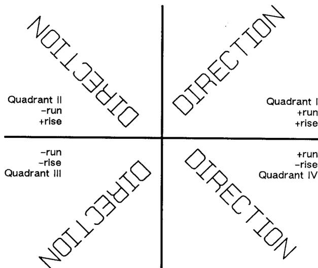
**Figure 23-19 Varying Print Direction with DI Command Parameter Sign**
