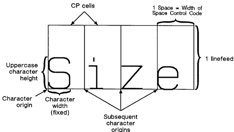
**Figure 23-8 Fixed-Spaced Font**
