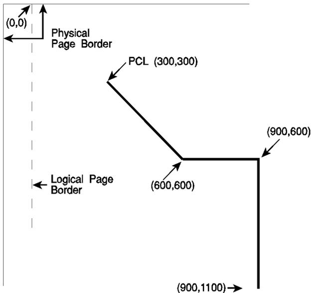
**Figure 19-10 Example: P1 and P2 command**
