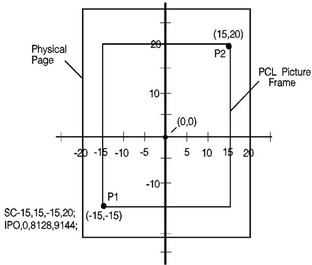
**Figure 19-3 New P1 and P2 User-Unit Scaling with Negative Values**
