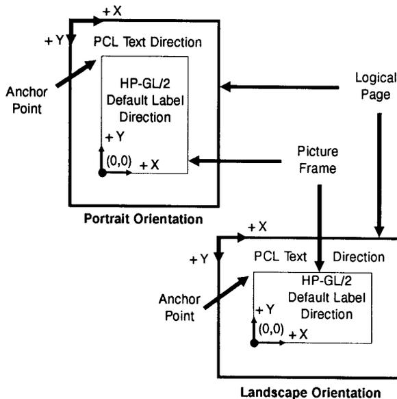
**Figure 17-6 Orientation Interactions Between PCL and HP-GL/2**
