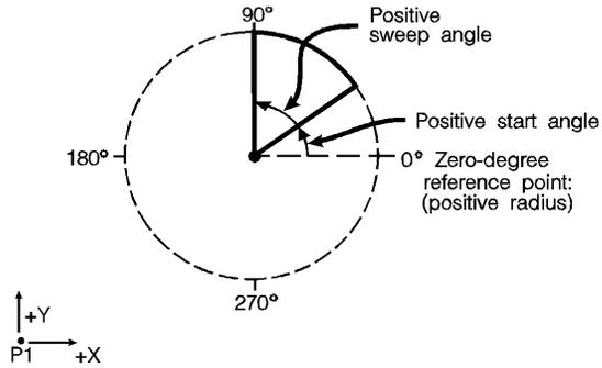
**Figure 21-4 Drawing Wedges**
