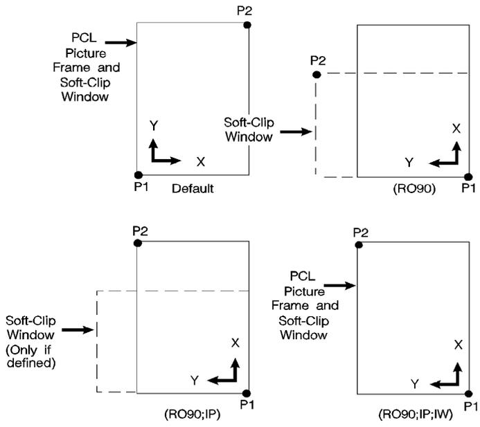
**Figure 19-17 Using IP and IW after the RO Command**
