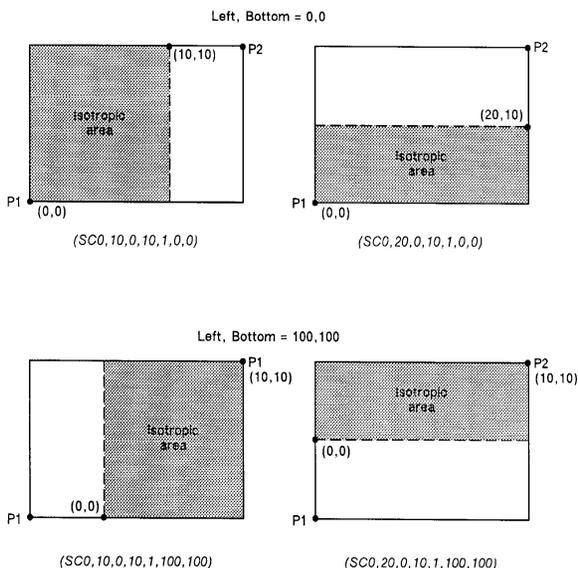
**Figure 19-19**The Left and Bottom Parameters
