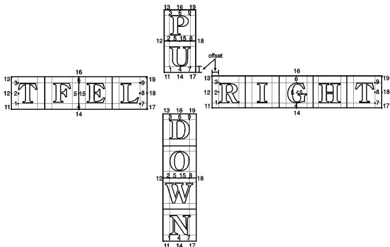
**Figure 23-33 Label Origin Positioning**
