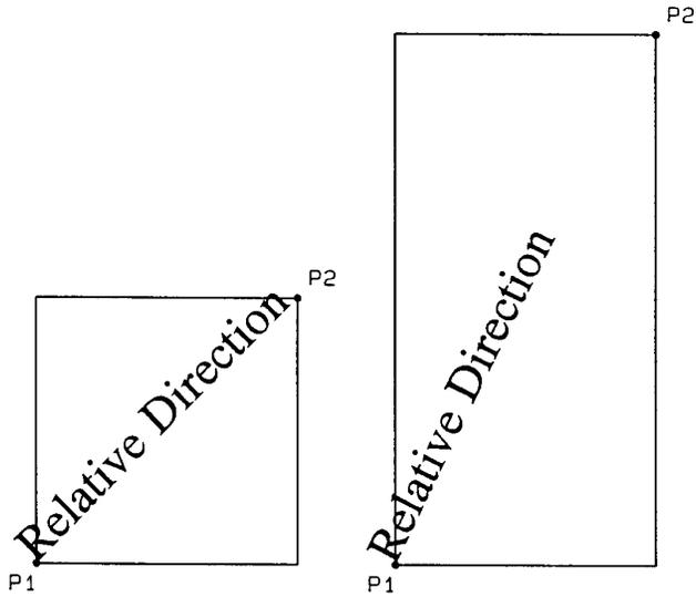
**Figure 23-23 Effects of Scaling on Label Direction**
