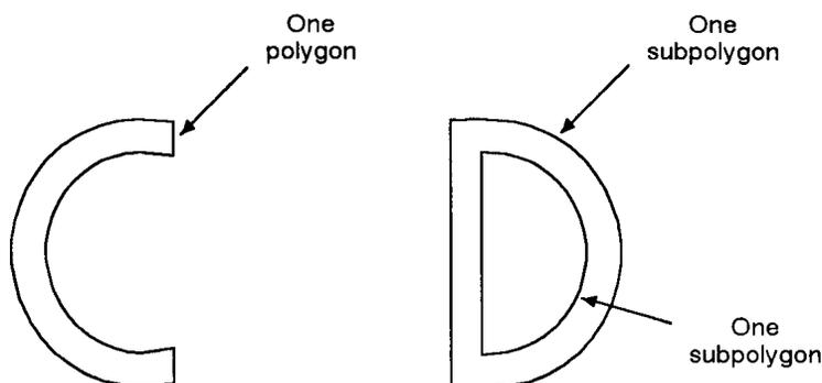
**Figure 21-7 Drawing Subpolygons**
