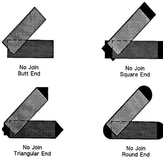
**Figure 22-13 Overlapping Line Ends without Line Join Selection**
