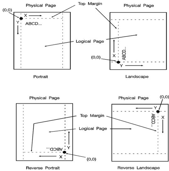
**Figure 5-1 Page Orientation With Default Print Direction**
