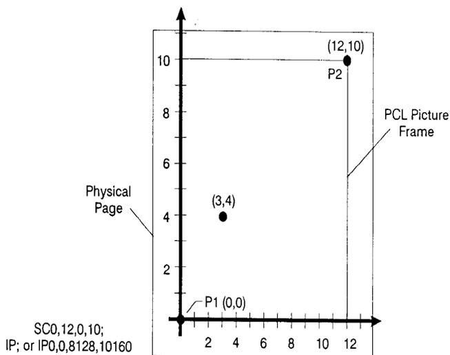
**Figure 19-1 User-Unit Scaling with Default P1 and P2**
